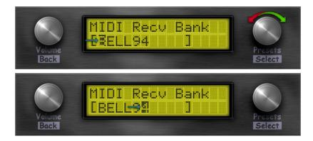
6. At the position where the letter is to be changed, the preset encoder must be pressed to switch to *edit mode*.
