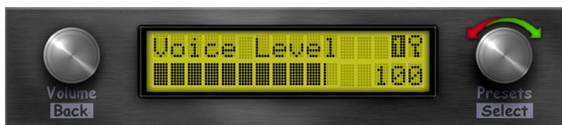
By changing (and later saving) this value you can compensate for differences in volume between different sounds. The value ranges from 0 to 127. Default is 100, but you can make the sound louder by increasing the value.
