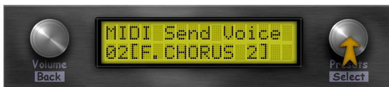
**Note on sending voice data:** The voice data is sent on the current MIDI channel. If the MIDI channel is *OMNI* the data will be sent on Channel 1.
