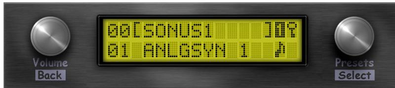
To switch between voice and bank selection, the preset encoder must be long-pressed.
