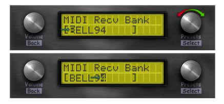
6. At the position where the letter is to be changed, the preset encoder must be pressed to switch to *edit mode*.
