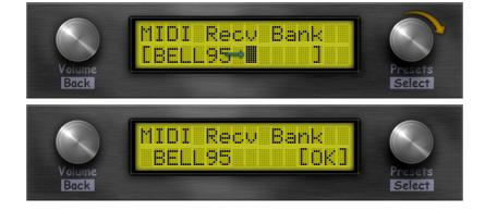
11. Push the preset encoder to wait for the data to receive.
