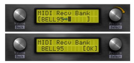
11. Push the preset encoder to wait for the data to receive.
