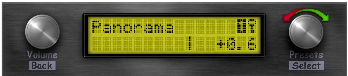
The place in the stereo image can be adjusted here (MIDI-CC 10)
