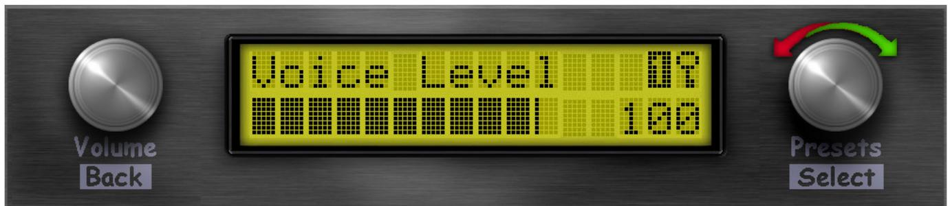
By changing (and later saving) this value you can compensate for differences in volume between different sounds. The value ranges from 0 to 127. Normal is 100, but you can make the sound louder by increasing the value.
