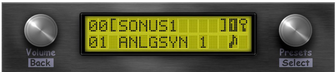
To switch between voice and bank selection, the preset encoder must be pressed for a long time.
